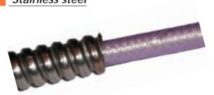
temperature range : - 65° C to + 165° C Crush resistance : 350 Kg / 772 Pound Min. bending radius : min. cable bending radius Flexible hose of stainless steel. This ruggedization protects the cable against compression, abrasion, mechanical injuries, open fire and hot objects (soldering irons for example). The continuous temperature is limited by the cable to +165°C, and in the immediate proximity of the connectors to the maximum connector temperature.
